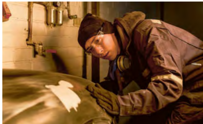
Above: First, Carlos Tapia checks how level the putty is before starting sanding.
