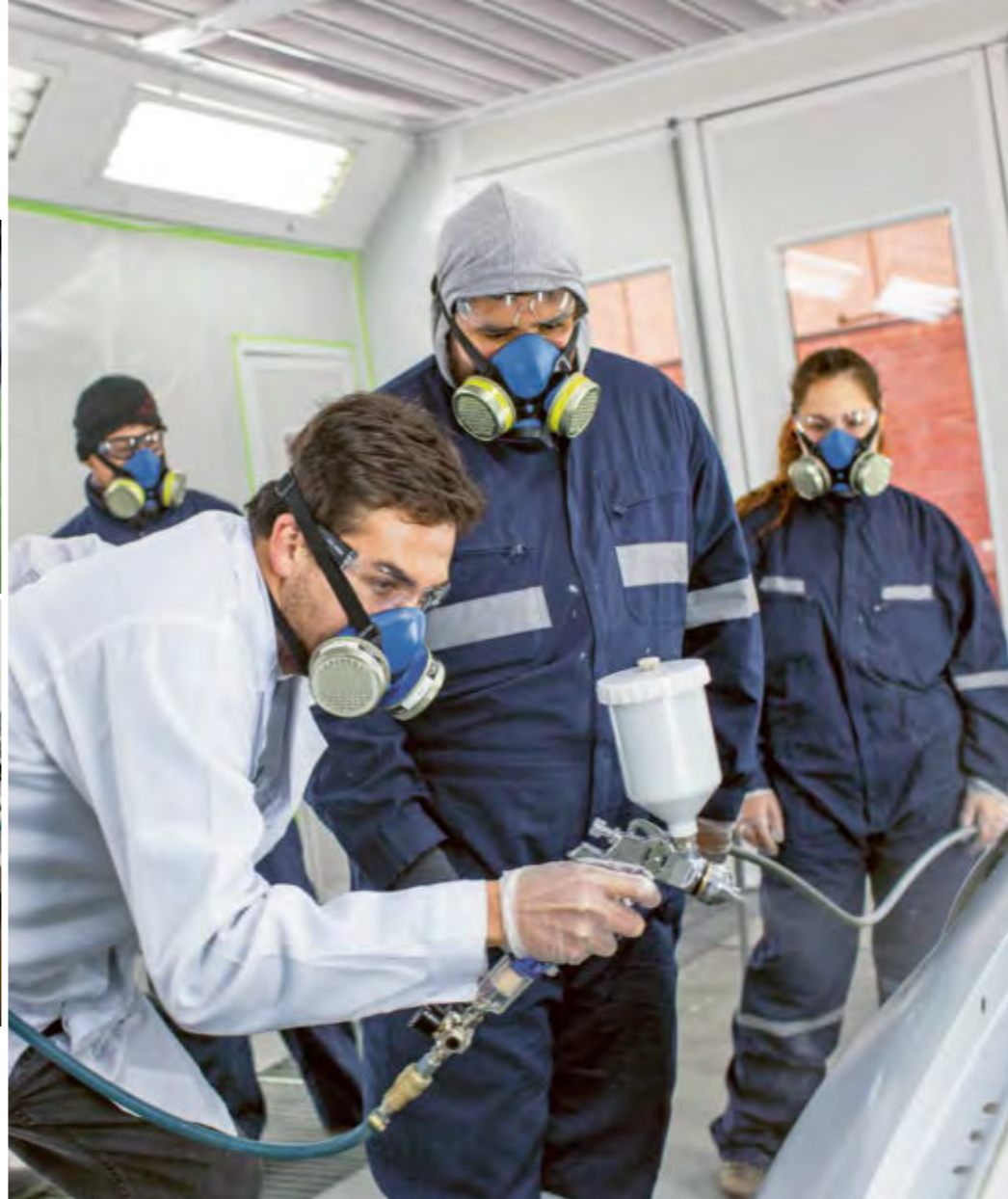
Above: Cristóbal Alvarado shows Michel Arce and Trinidad Chaparra how to evenly apply primer.
