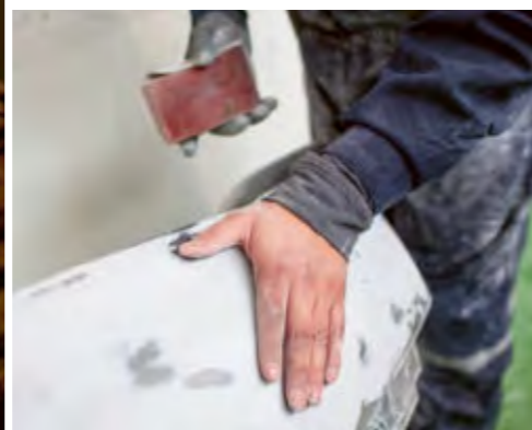
The car panels are filled with putty and sanded down ready for painting with filler and primer.
