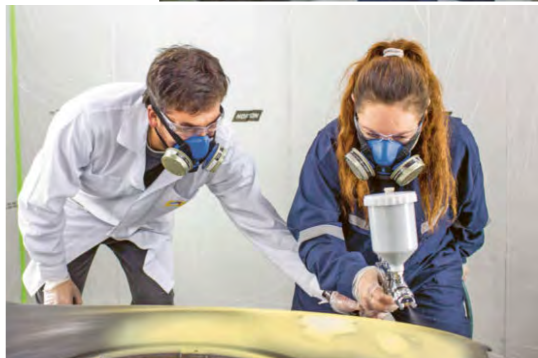
Above: Cristóbal Alvarado shows Michel Arce and Trinidad Chaparra how to evenly apply primer.
