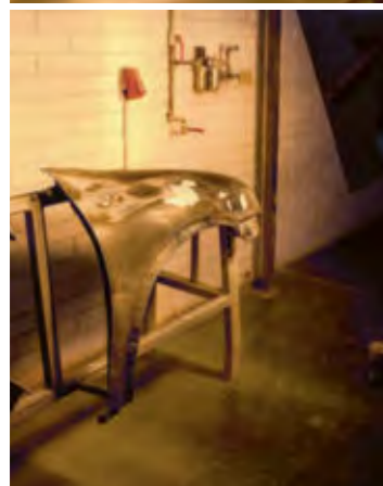
Next, the panel is put under a heat light to dry the putty.
