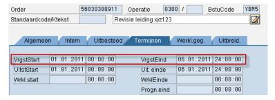
This change is automatically forwarded to AVISOR and is later also visible in AVISOR under "start execution" and "end of execution":
