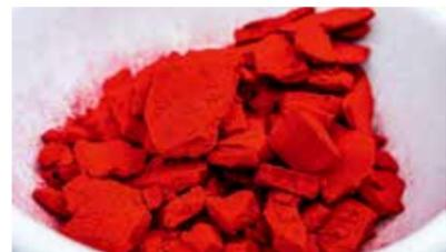
A few grams of a red DPP-based color filter pigment immediately after synthesis in the lab. The pigment is produced by the ton following a production scale-up.
