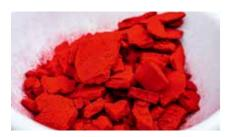
A few grams of a red DPP-based color filter pigment immediately after synthesis in the lab. The pigment is produced by the ton following a production scale-up
