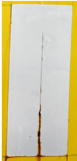
987 hours of ASTM B-117 salt spray at 2 mil DFT
