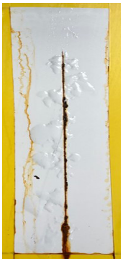
987 hours of ASTM B-117 salt spray at 2 mil DFT
