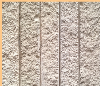
Different bubble structures of gypsum wallboards
