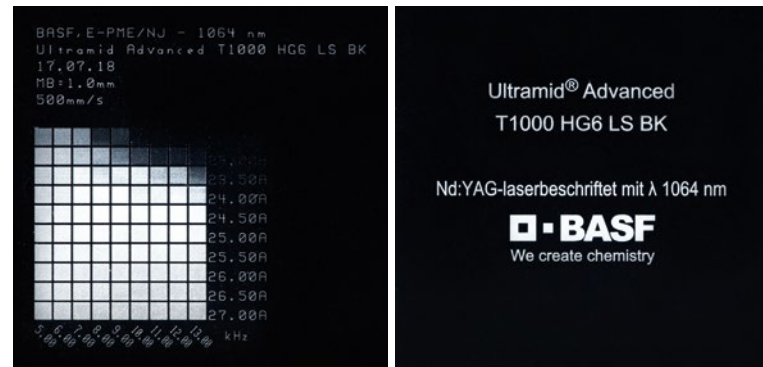
Fig 9: With Ultramid® Advanced T1000, parts can be excellently laser-marked.
