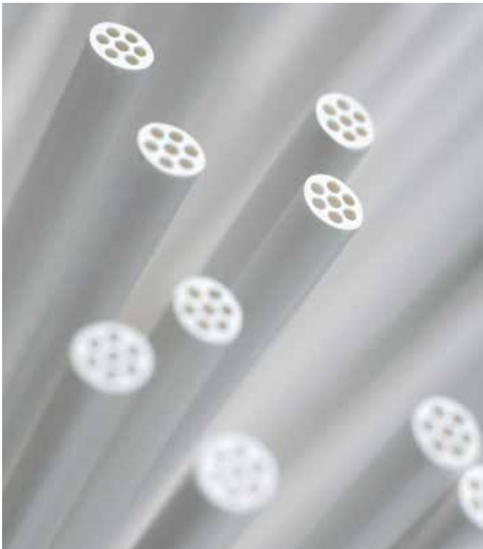
Cross-section through the filtration fibers: The honeycomb-like arrangement of the seven capillaries stabilizes the fibers. In this way the membranes are protected from fine cracks through which disease pathogens could penetrate. (Photos: BASF)
