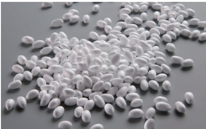
The individual Infinergy® beads have a size of from 5 to 10 mm and are supplied with a bulk density of approximately 110 kg/m³.
