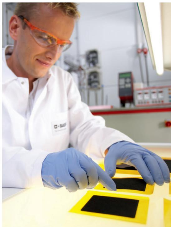
BASF has been manufacturing the Celtec® membrane since 2005. In a global network with science and partners, BASF has continuously adapted the membrane properties to the varying requirements of hydrogen separation and fuel cells. The membrane is produced by a sol-gel process.
