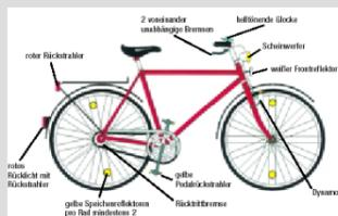
Clockwise starting from top left: Red rear reflector, 2 separate brakes, high-pitched bell, lamp, white front reflector, dynamo, amber pedal reflectors, back-pedal brake, amber spoke reflectors (at least 2 per wheel), red rear lamp with reflector
