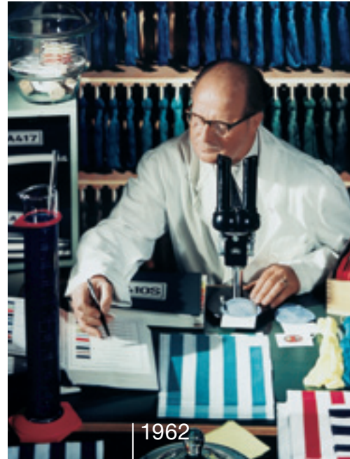
Determining the color and color strength of textile dyes
