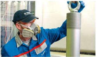
The functional coating contributes to the compliance with new emission limits. By coating the spindle in high pressure valves the friction in the thread, and particularly at the packing gasket, is reduced. Thus, a higher surface pressure can be realized in the packing which results in significantly lower leakage rates. This enables, in many cases, the adherence of environmental targets.
