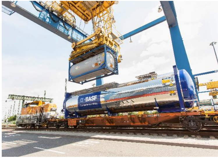
Standard tank container 25,000-36,000 liter volume 25 tons payload
