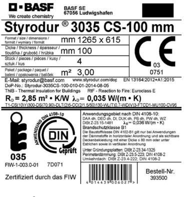
Styrodur<sup>®</sup> label with KEYMARK and "DIN-Geprüft" (DIN-Tested) logo
