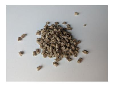
As an additive for industrial materials such as plastic, rubber, and concrete, Heartland's Imperium Masterbatch, a product designed to be blended with polymers, enables the production of high-performance natural fiber products and packaging.
