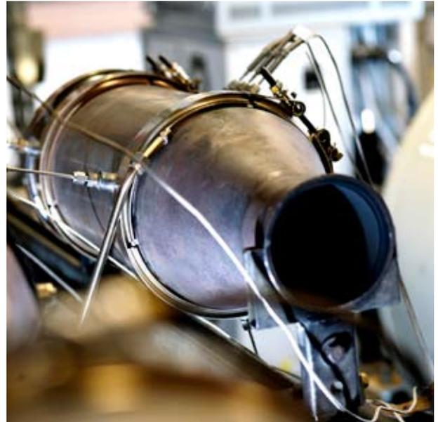
Vehicle catalysts are tested under long-term conditions at BASF's catalyst testing facility in Union, New Jersey. Complex electronic sensors are used to record all exhaust gas values during testing. The experts at BASF Catalysts are among the leading innovators in the development and optimization of catalysts for gasoline and diesel engines.
