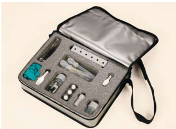
A spot test kit developed by BASF allows food producers to check the concentration of the vitamin during the food fortification process.
