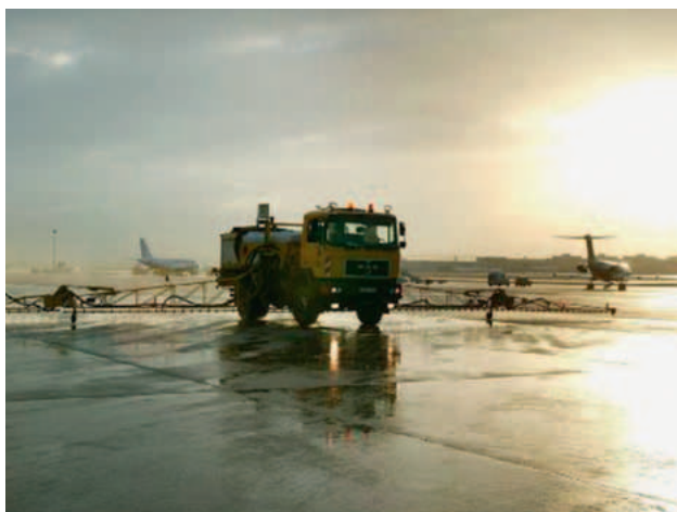
Using formates to de-ice runways: Very environmentally friendly, formic acid salts are effective in removing thin sheets of ice.
