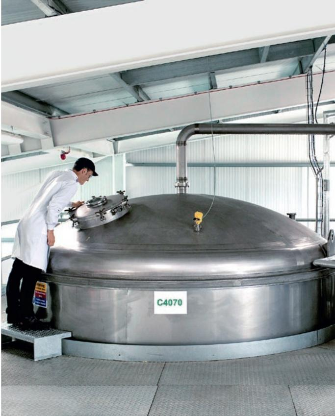
At its site in Littlehampton, BASF breeds nematodes in a 102,000-liter fermenter tank, spanning several levels.
