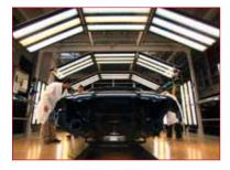
Final check in the varnishing line: the clearcoat as uppermost layer protects the automobile from external influences. With the clearcoat iGloss a car looks as good as new for longer.
