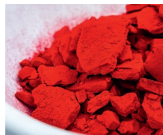
A few grams of a red diketopyrrolopyrrole-based color filter pigment immediately after synthesis in the lab. The pigment is produced by the ton following a production scale-up.
