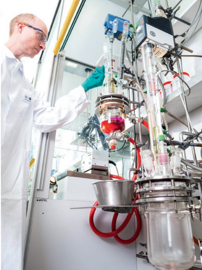
The picture shows a chemical reaction in the lab yielding diketopyrrolopyrroles, the substances BASF’s red filter pigments are made of. Diketopyrrolopyrroles are aromatic organic ring compounds mainly consisting of carbon, nitrogen and oxygen.
