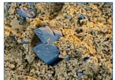
Nanoscale crystal seeds also make concrete harden faster at normal outside temperatures (magnification 960:1 at 12 cm image width).
