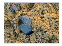
Nanoscale crystal seeds also make concrete harden faster at normal outside temperatures (magnification 960:1 at 12 cm image width).
