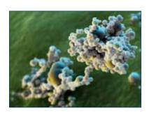
Their perfect spherical shape makes the particles of carbonyl iron powder from BASF particularly suitable for use in electronic components such as high-frequency coils.
