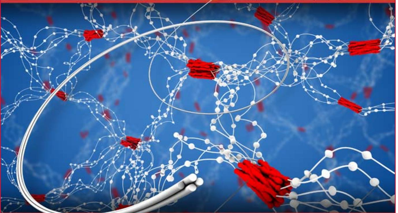
Spandex fibers can be stretched to seven times their length. Two different segments are responsible for this effect:
