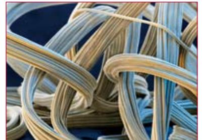
The basis of these fibers – consisting of several filaments – is PolyTHF.
