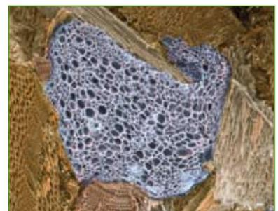
*Foamed polymer fills the cavities between the wood chips, generates counterpressure and, by creating additional binding sites, provides high strength.*
