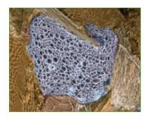
Foamed polymer fills the cavities between the wood chips, generates counterpressure and, by creating additional binding sites, provides high strength.
