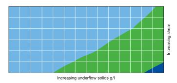
The Rheomax® DR range of products produce an underflow with a lower yield stress, which is more tolerant to fluctuations in solids content and applied shear, resulting in a more consistent thickener performance over a wide range of operating parameters.
