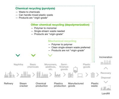
Chemical recycling can help recycle post-consumer plastic waste streams that would otherwise end up in landfill or be used for energy recovery. Examples are plastics with residues or mixed plastic waste fractions, consisting of different plastic types, which are not suitable for further sorting.
