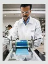
Laboratory for polymer additives and pigments in Mumbai, India Preparing a sample to determine the suitability of a BASF pigment used for printer ink.
