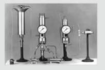
**Experiment apparatus** Small equipment, great effect: the apparatus of Fritz Haber (shown here in a replica) lays the foundation for BASF's ammonia synthesis on a small scale.
