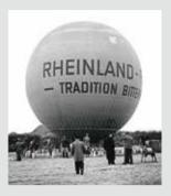
Air measurements with halloons In 1960, BASF chooses an exceptional method to measure air values by using an open-air balloon. In contrast to machinepowered aircrafts, a measuring balloon allows faultless air measurements. Two plastic tubes with a length of 400 meters suck in the air to be measured.
