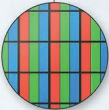
Each individual pixel is composed of red, green, and blue subpixels that can be switched on and off, one by one.
