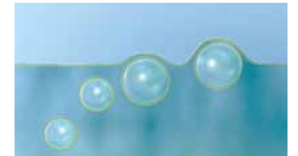
Figure 2: Orientation of surfactant molecules around foam bubbles. Foam bubbles on top of a liquid exhibit a surfactant double layer around the foam bubbles.
