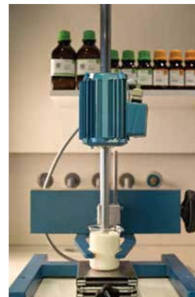
Figure 7: Dissolver and pycnometers to determine density after stirring.
