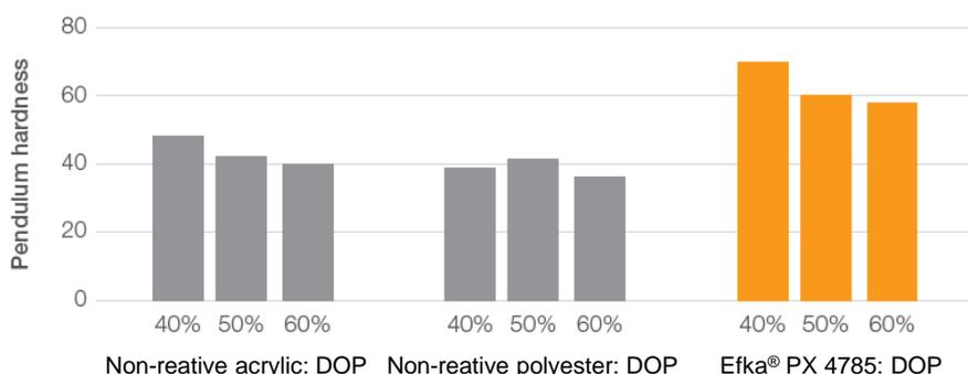
Efka® PX 4785 provides highest pendulum hardness (Irgazin Red / PR 254 paste formulation)
