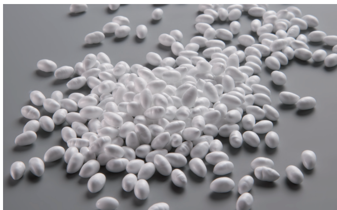
The individual Infinergy™ beads have a size of from 5 to 10 mm and are supplied with a bulk density of approximately 110 kg/m 3 .
