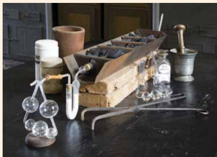
Above The “five-bulb apparatus” is made out of the finest glass and is filled with concentrated potassium hydroxide. In a short period of time it collects carbon dioxide created during combustion so that it can be weighed on an analytical balance. With this invention, Justus von Liebig revolutionized elementary analysis.
