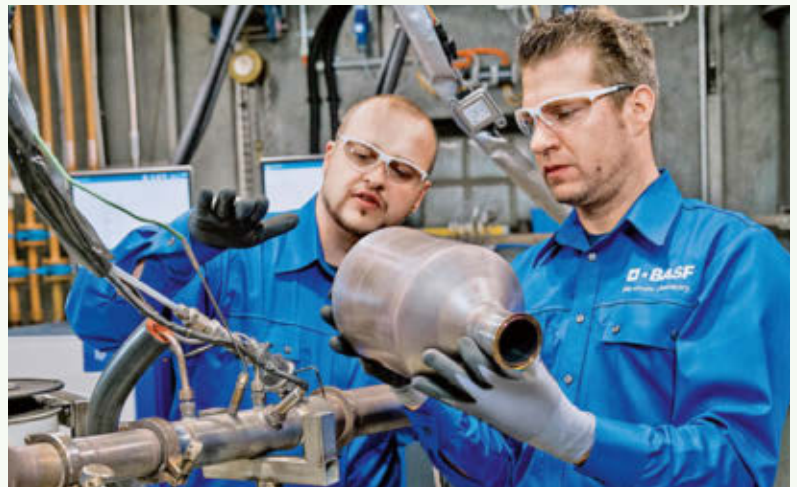
At BASF's Hanover Engine Lab, future catalyst technologies are tested for their functionality and durability.
